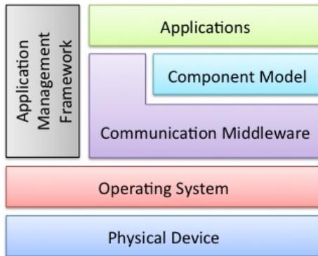
Fig. 3. Overview of target system architecture.
