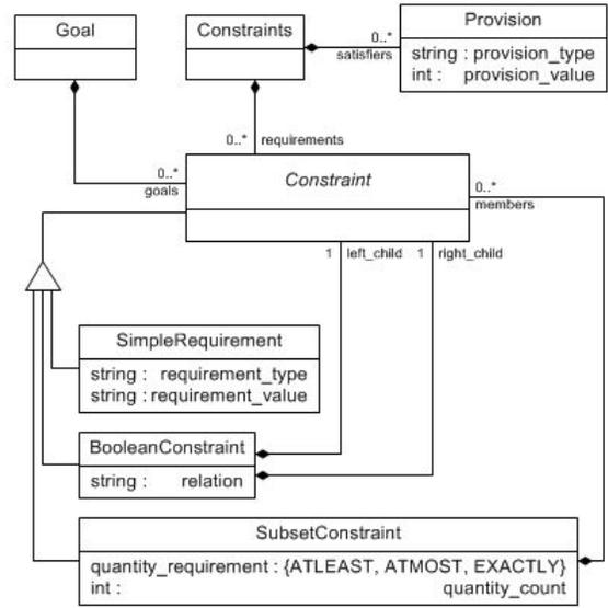
Fig. 7. UML class diagram for Constraint category.
