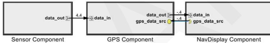
Figure 9: Example: Component Interactions. Here each interface is annotated with its (periodicity, deadline) in seconds.
