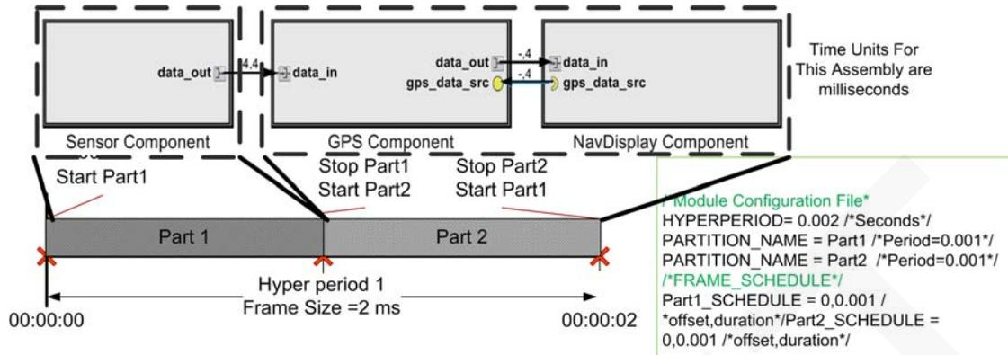
Figure 12: Software Assembly and Deployment Diagram used in the case study.
