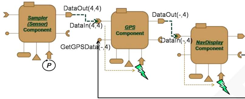
Figure 5: Example: Component Interactions. Here each interface is annotated with its (periodicity, deadline) in seconds.
