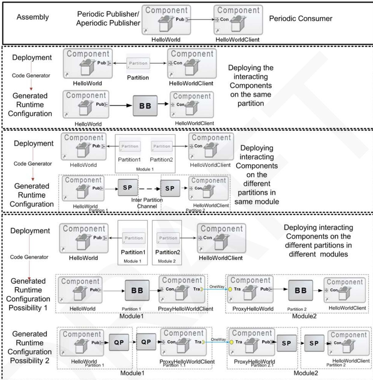
Figure 11: Same interaction results in different runtime configurations based on deployment. This is done by the code generator, freeing the system developer to focus on the application logic instead.
