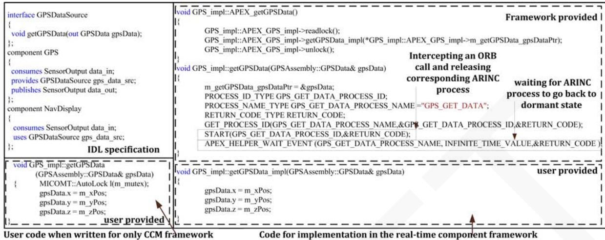
Figure 10: Equivalent implementation of a CORBA CCM interface in our ACM framework.
