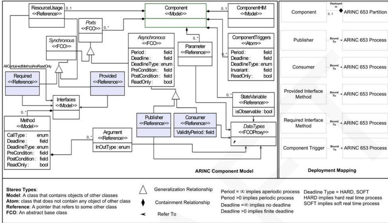
Figure 4: ACM Metamodel. The colored boxes indicate the four types of ports, which can be used to interact with other components.
