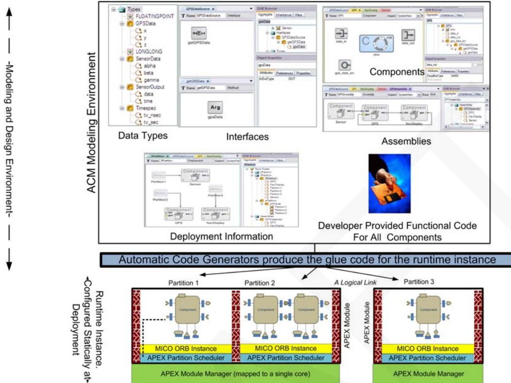
Figure 8: The system architecture, component configuration, correctness contracts, assemblies are specified in a domain specific modeling language. This model is used to generate an instance of executable assembly.
