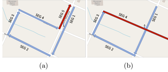
Fig. 2: (a) Overlapping segments. Segments 1 and 5 traverse the same section in opposite directions. (b) Intersecting segments. Vehicle locations near the intersection of segments 1 and 4 can lead to incorrect mapping. Stops not shown.
