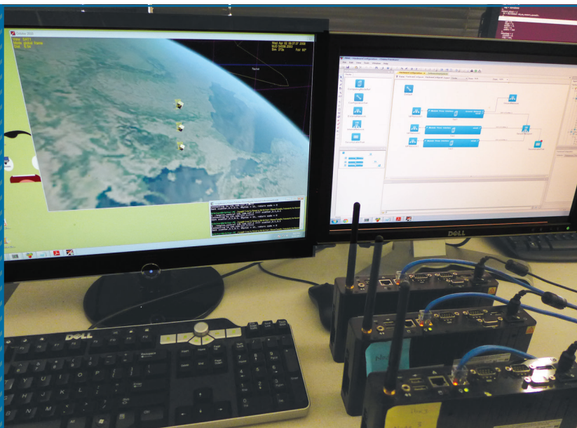
FIGURE 4. The runtime platform's deployment. The simulator image (on the left) shows three satellites, whereas the other display (on the right) shows the deployment model of the experiment.
