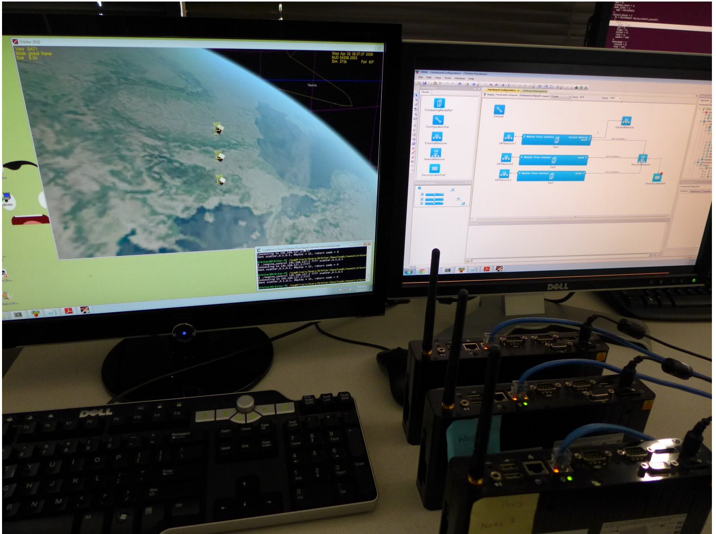
Fig. 2. Development system and DREMS cluster : The bottom right of the image shows the 3 computing nodes used for this application deployment; the left screen shows their three corresponding satellites simulated in orbiter (which is communicating with the three nodes); and the right screen shows the application development using the modeling tools.
