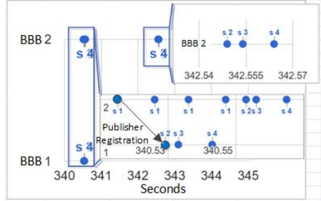
Fig. 6. The plot here has two Beaglebones on the y axis. The points denote the events (s1-s4) for each Beaglebone when BBB2 rejoins the cluster. The two zoom in boxes show the events in detail as they happen on timescales on the order of milliseconds. At the beginning of this test two nodes were started. After some time BBB2 was rebooted. In the zoomed box between times 340 and 341, the first event shown is s1 for BBB2 when it registers its publisher service. The s2 event for BBB1 is when BBB1 receives the notification of BBB2's service 14ms after BBB2 registers it. 4 and 10ms later BBB1 notifies it's requesting component and that component connects to the publisher respectively. Towards the end of the first zoom in box we see s2, 3, and 4 events when BBB2 receives notification of its own service. The second zoom in box between 342 and 343 seconds shows BBB2 again receiving notification of its own publisher. Covered by the second zoom in box at 344.5 seconds BBB2 finally receives notification of the publisher on BBB1. There is some behavior where a new node receives notification of the first service it discovers twice.
